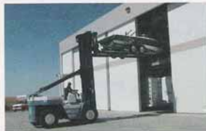
A boat on a trailer is lifted to a rack at Gold Key Boathouse. Notice how the side doors slide open for depositing the boat and trailer.
