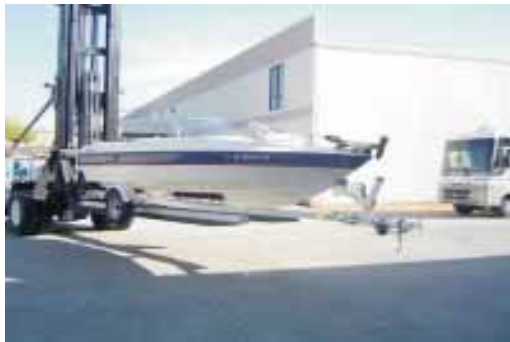
Marine forklift with boat & trailer
