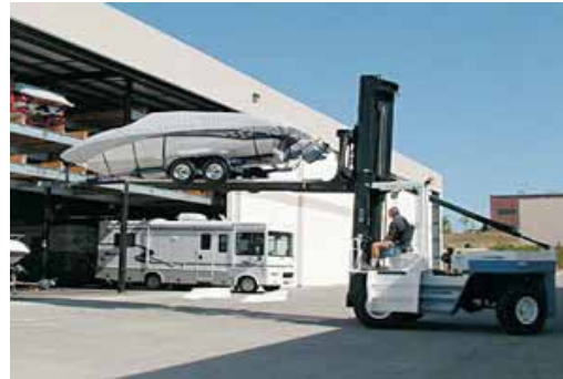
Marine forklift with boat & trailer - 2nd level
